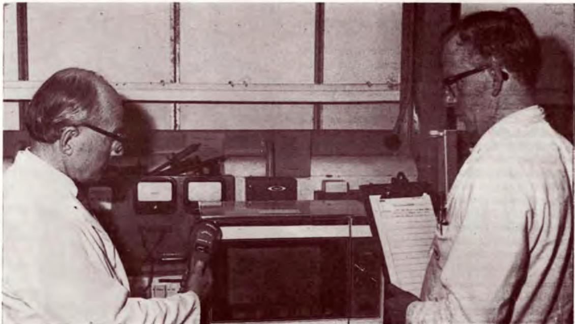
Test engineer Tom Owen, left, assisted by John Whittle, checks a microwave oven for leakage, with negative results.
