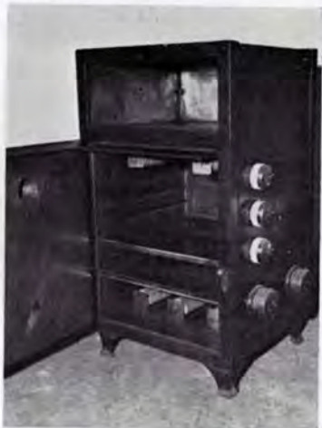
One of the first electric cookers with oven heating elements each controlled by its own switch.
